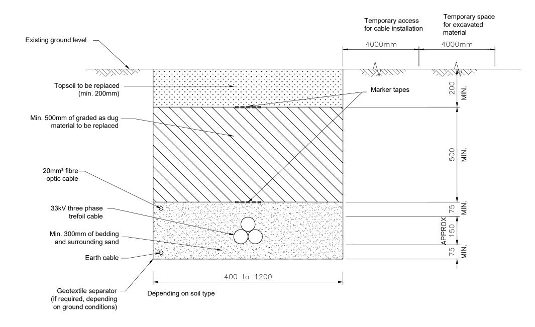
Typical Cable Trench Detail (typically adjacent to road) 1:10 @ A3
